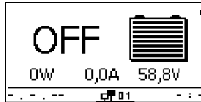
Fig. 7: Display after switching on the external battery fuse
