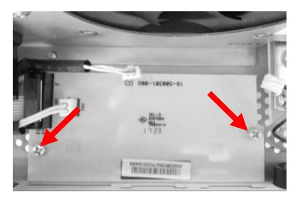
Figure 4: Remove screws on beige board
