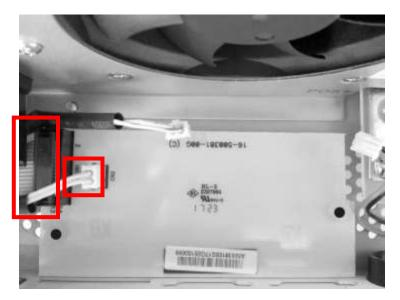
Figure 5: Remove connectors on beige dummy board
