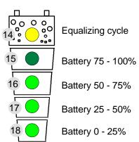
This means that the display can, within few minutes during the charge, commute from 25% to 75% or during the discharge, to the opposite direction.
